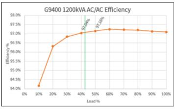
G9400 1200kVA UPS with 42% load efficiency = 97.08%
