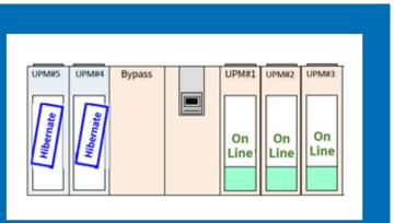
Here is a scenario of how the selectable High Efficiency Hibernate (HEH) feature functions on a Toshiba G9400 2000kW UPS:
